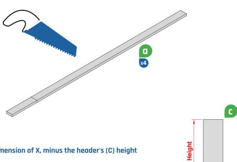
Cut verticals (A) to the dimension of X, minus the header's (C) height
