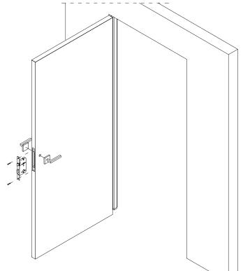
It is most important that you install your lock into the door at the exact height to suit your strike plate. REMEMBER, the adjustment on the hinges is there to adjust slight irregularities of the frame installation and will not compensate for any lock mis-positioning. You are responsible to ensure the lock is installed at the correct position, the adjustable hinges are there only to adjust the door panel relative to the frame.
