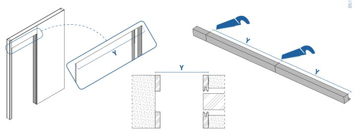
For 35 mm Doors - Cut brushes (**D**) to dimension **Y** and insert into both headers (**C**)
