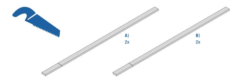
If the framework is not installed at finished floor level then cut  $\bf A$  and  $\bf B$  as shown below  $\bf X=41$  mm.
