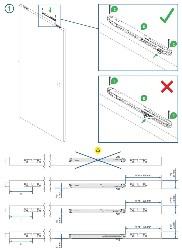
For doors of 26" (660 mm) or smaller, place X at 3 1/8" (80 mm) from the door's rear edge.
