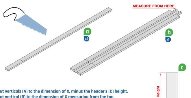
Cut verticals (A) to the dimension of X, minus the header's (C) height. Cut vertical (B) to the dimension of X measuring from the top.
